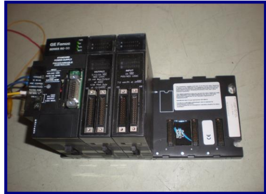
GE Fanuc Series 90-30 PLC Simulator
