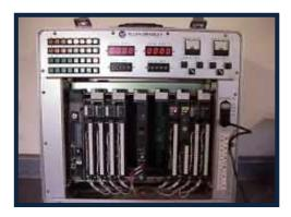
Allen Bradley WS5610 PLC Simulator PLC5
