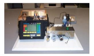
Ultrasonic Testing (UT) Equipment
